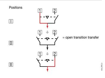
SOCOMEC transfer switching equipment is designed as open transition that meets the requirements for most applications. In fact for most applications the backup supply is rarely a hot standby (example a genset needs to be started) whilst critical loads are usually supplied through a UPS.
