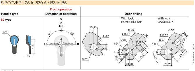
(1) Ø31 to Ø37: rear screw mounting, Ø37: front clip mounting.
