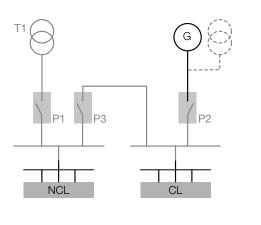
Second type of architecture: S1 (kVA) > S2 (kVA)
