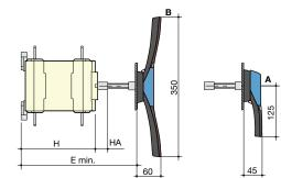
A. S2 type handle for external operation: 125 to 630 A B. S4 type handle for external operation: 800 to 1600 A
