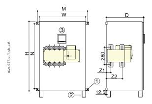
(1) Wall mounting brackets supplied up to 400 A.
