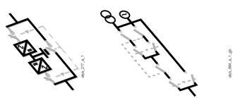
Isolation of the a transfer switch, a UPS or other equipment for scheduled maintenance or tests. This is done by safely disconnecting upstream and downstream circuits, whilst continuing to supply the load via a parallel circuit referred to as a Bypass circuit.
