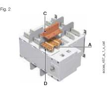
(1) Choose the bolt length according to the thickness of the bars being connected; if bar thickness is greater than 20 mm, 45 mm bolts are required.
