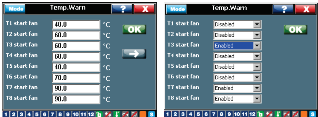
Figure 43: RVT temperature warning settings
