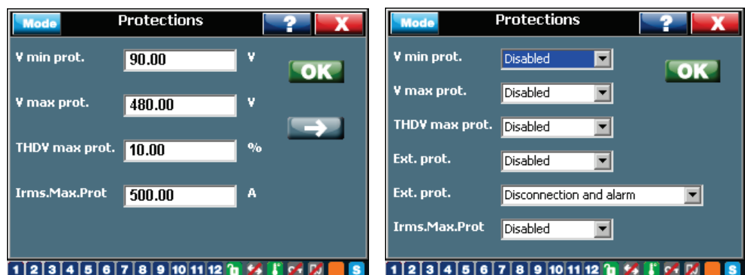
Figure 40: RVT protection settings
