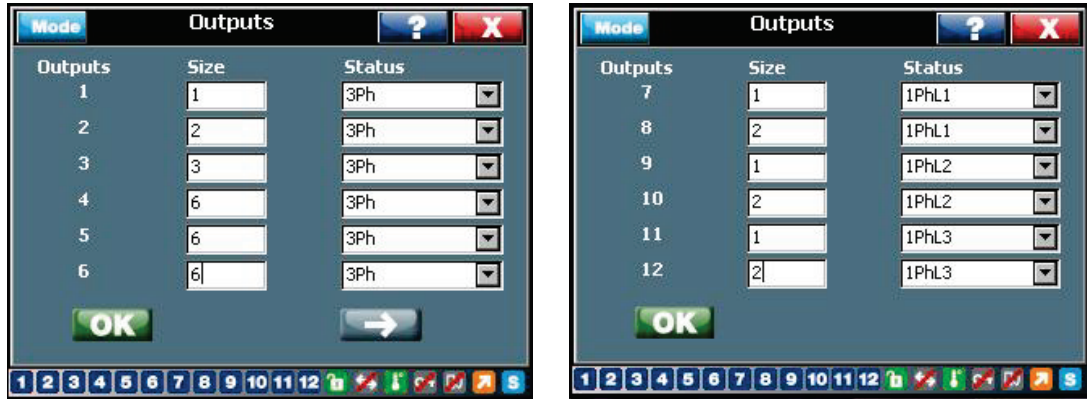
Figure 31: Typical outputs setting 6 x 3ph + 6 x 1ph (Three phase model RVT12-3P)
