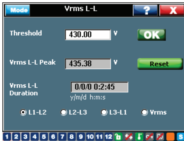
Figure 24: Event logging threshold setting - Vrms
