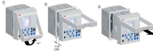
Figure-16 Removal of RER615 from it's case
