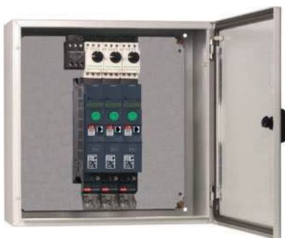
Example of GV2/ATV320 direct mounting in an enclosure: GV2L circuit-breakers + GV2454 and GV2G05 accessories + ATV320U18N4B drives
